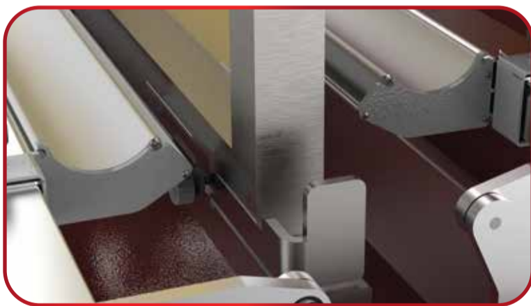
Screen holders are adjustable to accommodate a wide variety of frame sizes and thicknesses
