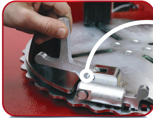
Self-centering clamps lock easily to keep containers in place
