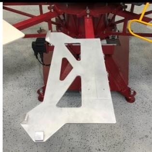
**4.** Move the registration pallet into position, pull the screen towards you. When contact is made with the guide pallet's three registration points, lock the screen in place. Repeat for all screens.
