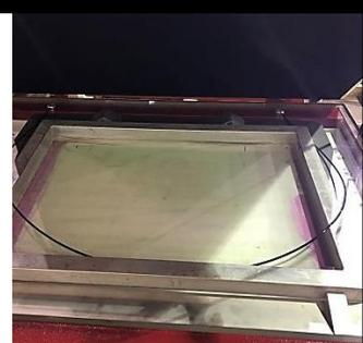
**3.** Mount the guide pallet on your press. The guide pallet replicates the registration points on the master frame, ensuring your films are aligned the same on press as they were on your exposure
