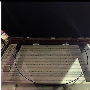
**2.** Place your screen into the master frame. The spring-loaded pins keep the screen and film tightly locked into place exactly against the registration points during vacuum drawdown.
